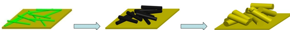
Figure 4.1. Computer schematic showing (1) virus assembly on chip, (2) virus particles after nickel coating, and (3) virus particles after gold coating
